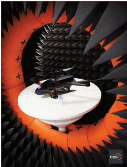
▲ Fig. 9 MVG's multi-probe system testing a drone.
