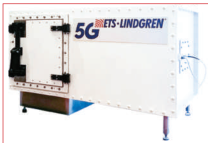
▲ Fig. 7 ETS-Lindgren's table top AMS-5700 OTA test chamber.
