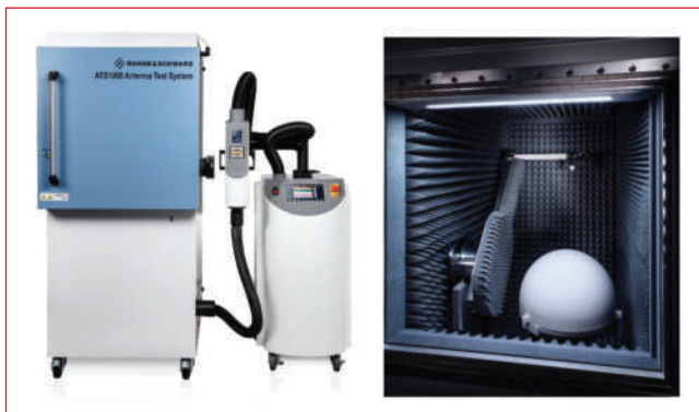
▲ Fig. 14 R&S ATS1000 test chamber.
