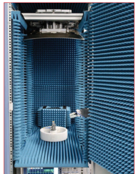
▲ Fig. 13 R&S ATS800R compact test chamber.
