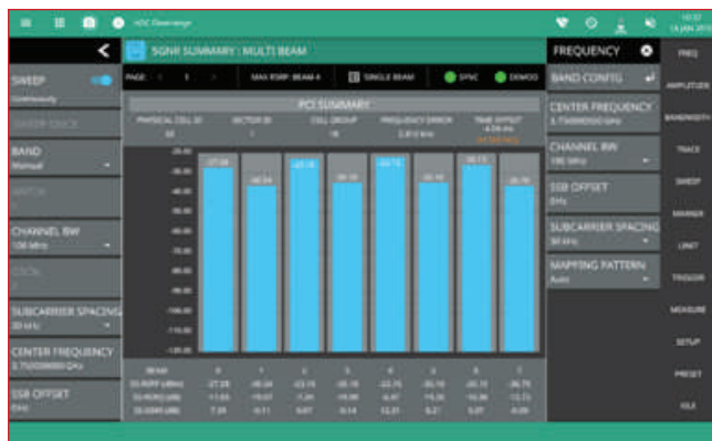
▲ Fig. 2 The summary screen displays all measurement results to validate 5G base station performance.
